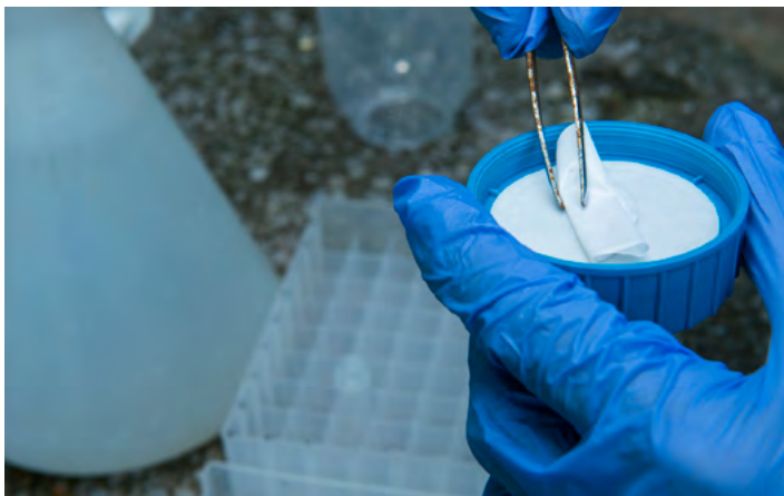
Fig. 5: Folding filter after filtration to store in tube with ethanol for later extraction and qPCR analysis. Photo: Pete Oxford.
