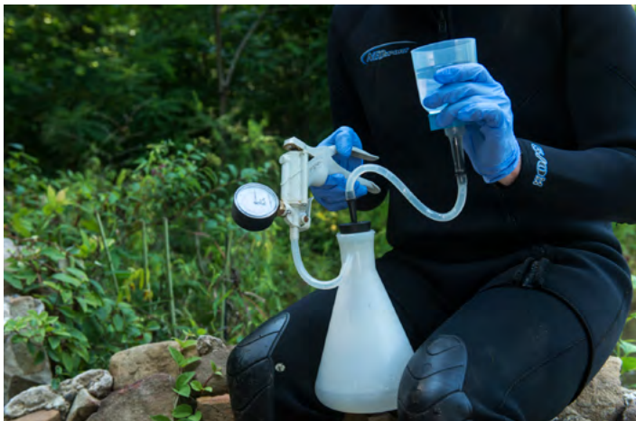
Fig. 4: Filtering water for eDNA. Water is collected and poured into a cup with a filter on the bottom, and then pushed through the filter using vacuum filtration. Photo: Pete Oxford.
